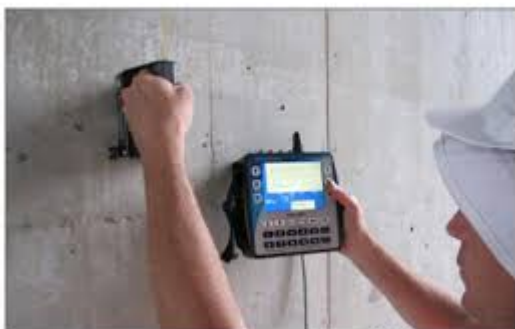
Impact Echo Testing Using Olson's NDE360
